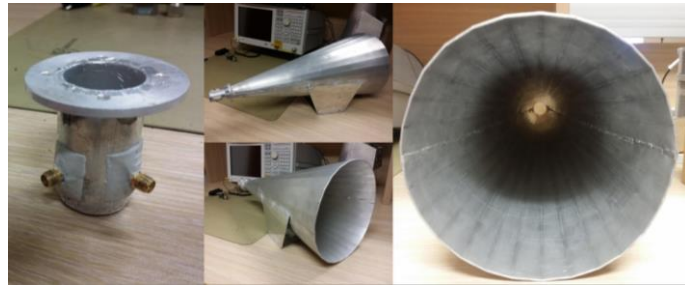
Figure 6: Prototype conical horn with dual polarised waveguide.
