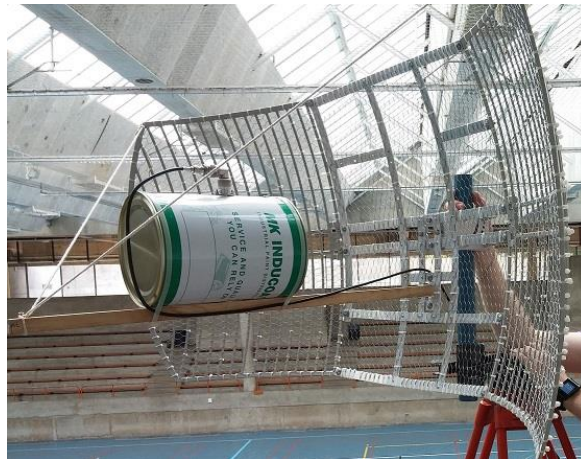
Figure 3: Prototype antenna with dual polarised waveguide feed mounted to a tripod for testing.
